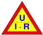
$$I_1 = \frac{U_1}{R_1} = \frac{220 \text{ V}}{400 \Omega} = 0.55 \text{ A.}$$
